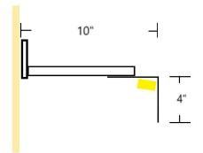
The RLX500-4S5 is a linear LED fixture with a 4"angle glare shield designed specifically for wall washing applications.
